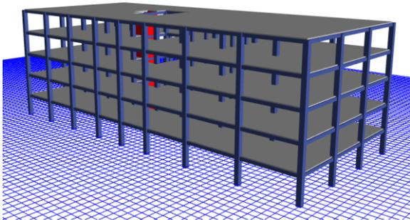
Fig. 1 3D model of commercial building modelled in ETABS2016
