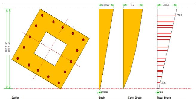
Fig.8 Stress and Strain diagram of results for hollow column in CSICOL9
