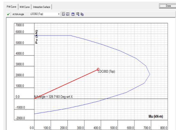
Fig.7 Interaction diagram of results for hollow column in CSICOL9
