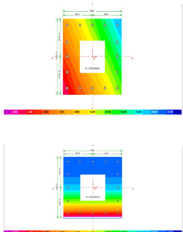
Fig.9 Stress variation diagram of results for hollow column in CSICOL9
