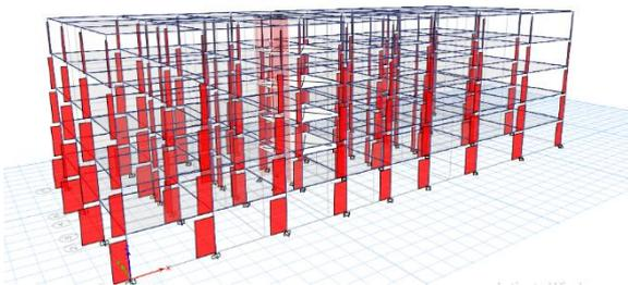
Fig.2 Axial forces acting on columns in ETABS2016
