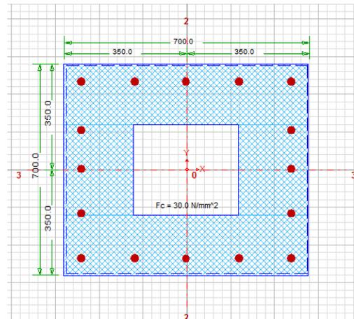
Fig.5 Cross section of hollow column in CSICOL9
