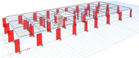
Fig. 3 Maximum values of axial forces acting on bottom story columns in ETABS2016
