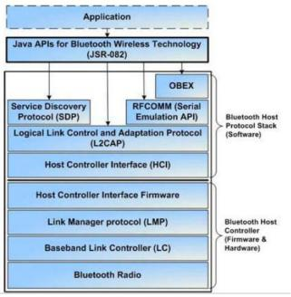
Fig 1:Bluetooth Stack with JSR-82
