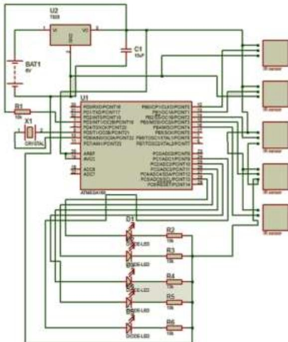
The above figure shows the circuit diagram of the given system. It consists of 5 LEDs along with 5 IR sensors.
