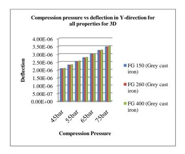
Fig.18: Compression Pressure vs. Deflection in Y-direction for all properties of materials for 3D
