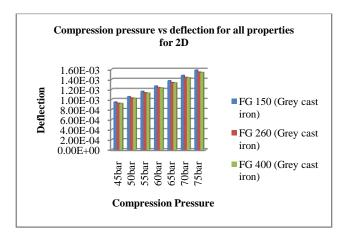
Fig.17: Compression Pressure vs. Deflection for all properties of materials for 2D
