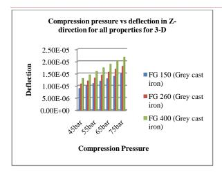
Fig.19: Compression pressure vs. Deflection for all properties of materials in Z-direction for 3D
