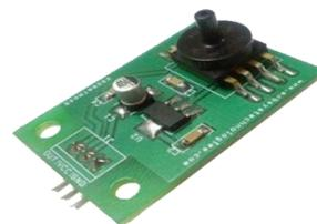
Fig. 4.c Blood pressure sensor
