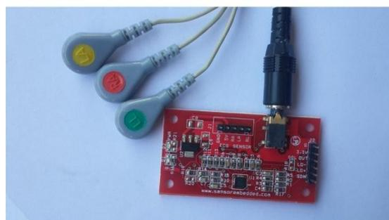
**Figure: 4.a ECG SENSOR**
