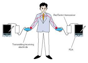
Fig. 4. Experimental setup for intrabody communication. **Fig 5.** Intra body Communication
