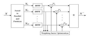
Figure 1 :PTS Block Diagram [3]
