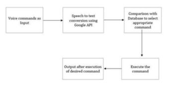
Fig. 1. Speech recognition block diagram
