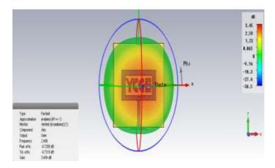
Figure 7: Gain of microstrip antenna with EBG at 2.486 GHz resonance freq.
