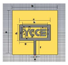
Figure 2: Patch antenna (Front view)
