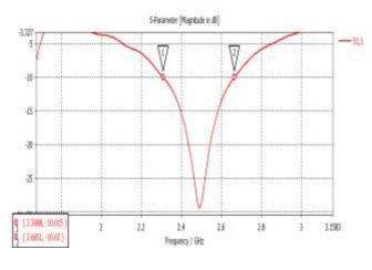
Figure 5: Simulated S-parameter result
