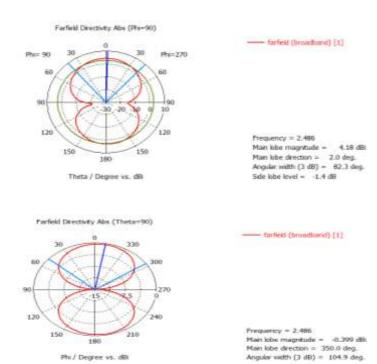
Figure 6: Radiation pattern at 2.486 GHz frequency.
