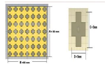
Figure 1: Design of EBG structure (a) Plus shape EBG substrate (b) EBG unit cell
