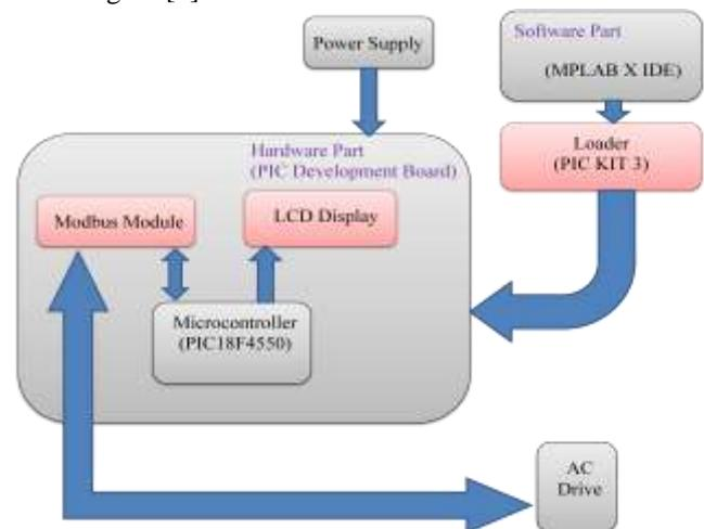
Figure 1: Block Diagram of Complete Project
