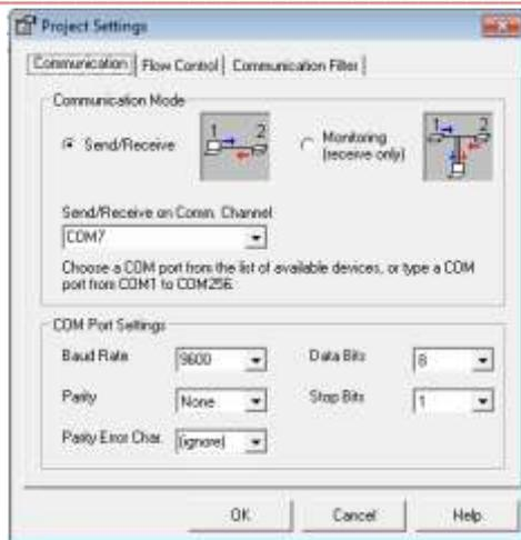
Figure 4.1: Project setting in Docklight Software
