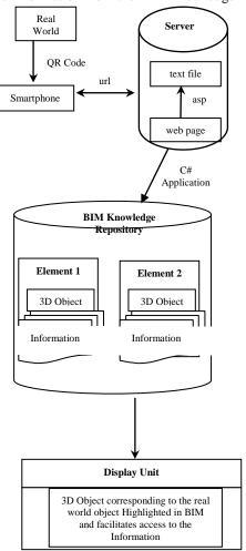
Figure 2: Automated information flow in BIM+QR environment
