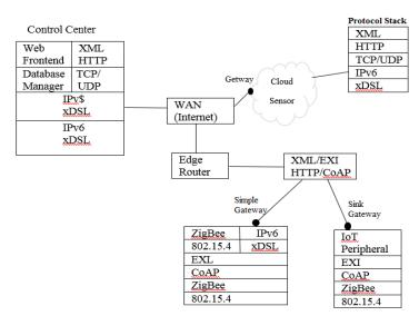
Fig. 2: System Block Diagram
