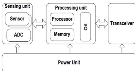
**Figure1.** Components of sensor node
