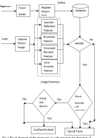
Fig.1 Block diagram of the proposed cascade structure for detection of spoofing face and medium
