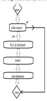
If the color sensing unit fails to identify the color of the note. The process stops there and the note is returned to the user via note placing unit.
