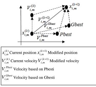
Figure 4: Concept of modification of a searching point by PSO
