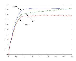
Figure 11: The step response after applying PPID on the Electro system
