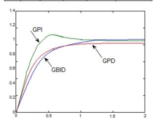
Figure 12: The step response after applying GPID on the Electro system
