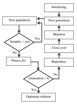
Figure 6. The optimization flowchart of GA technique.
