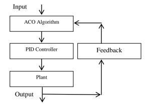
Figure 7. ACO-PID Controller
