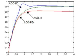
Figure 13: The step response after applying ACO-PID on the Electro system
