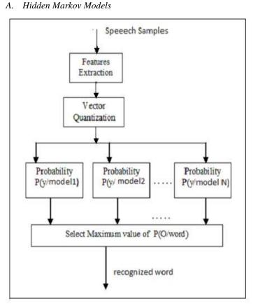
Figure 1. Recognition of spoken word using HMMs
