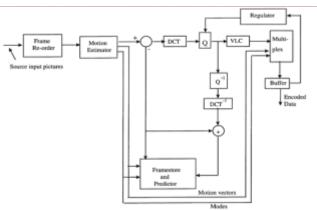
Fig.4 Block diagram of MPEG video encoder
