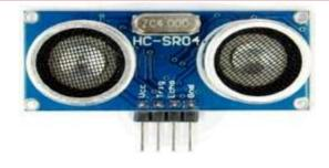
In Ultrasonic sensors, signal measurement is independent of material and color of obstacles. It works in all light conditions - bright, dark, glaring or dim. Suspended particles like dust, steam, smoke does not affect the measurements. HC-SR04 Ultrasonic Distance Sensor is a popular and low cost solution for non-contact distance measurement function. It is able to measure distances from 2cm to 400cm with an accuracy of about 3mm.
