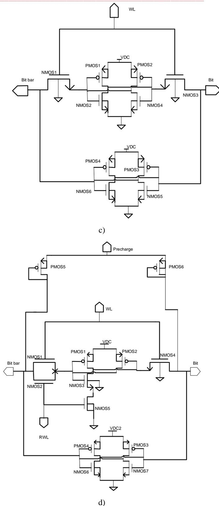
Figure 2. CMOS SRAM Cells a) 6T SRAM cell, b) 7T SRAM cell, c) 6T SRAM cell with cross-coupled invertors d) 7T SRAM cell with cross-coupled invertors.
