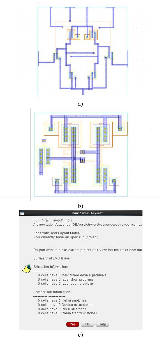
Figure 5. Layouts of SRAM Cells (CMOS 180nm) a) 6T SRAM cell b) 7T SRAM cell. c) LVS Report
