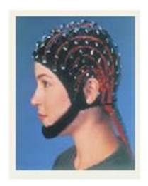
Figure 1: A subject wearing an EEG cap fitted with electrodes.
