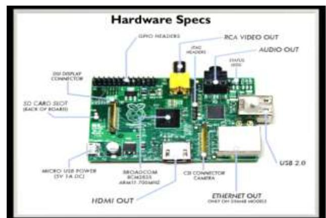
Figure 3: Raspberry Pi Development Board
