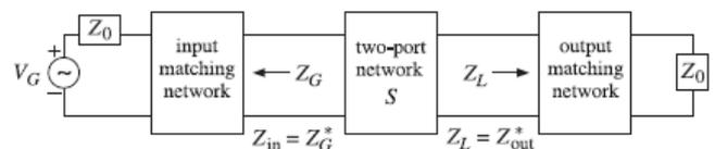
Fig.5. Impedance Matching Network
