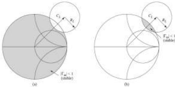
Fig.2. Output Stability Circles for a conditionally stable device
