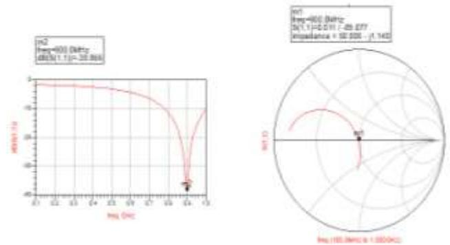
Fig.8. Response of input Matching network
