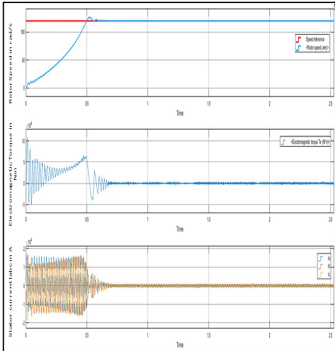
**Fig -6:** Performance of DFIM drive system when given reference speed is 120rad/sec at no load.
