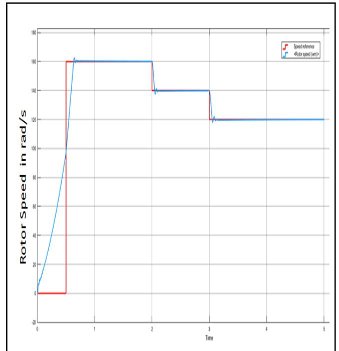
**Fig -8:** Rotor speed at variable reference speed condition.
