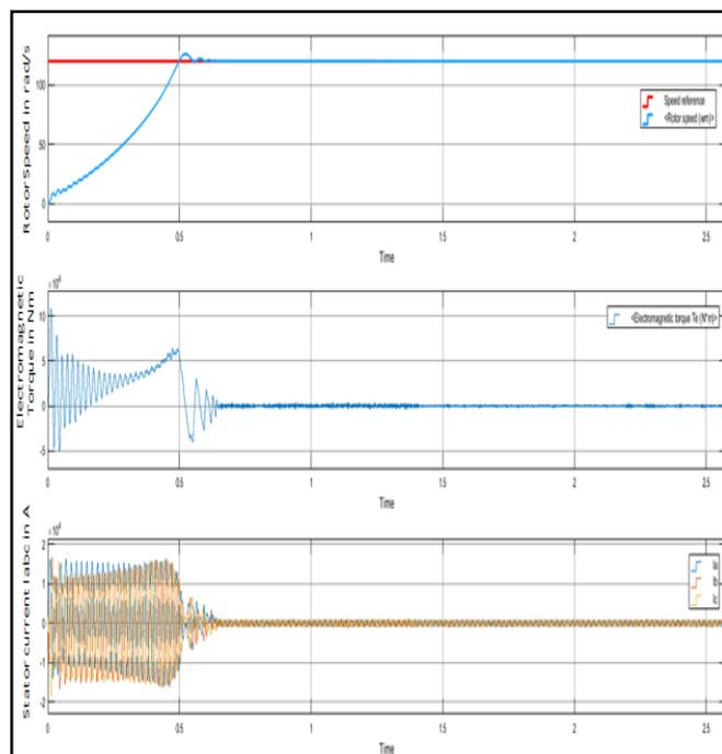
**Fig -7:** Performance of DFIM drive system when given reference speed is 120rad/sec at load 25Nm.
