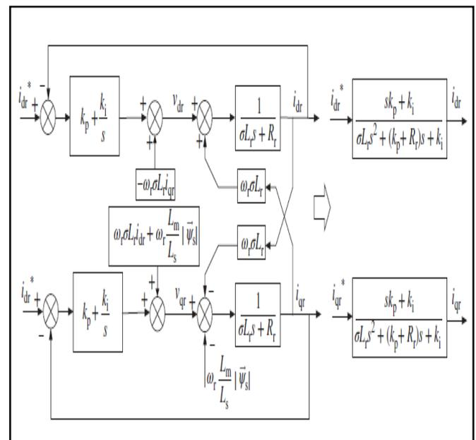
Fig-3: Equivalent second-order system of closed-loop current control with PI regulators.
