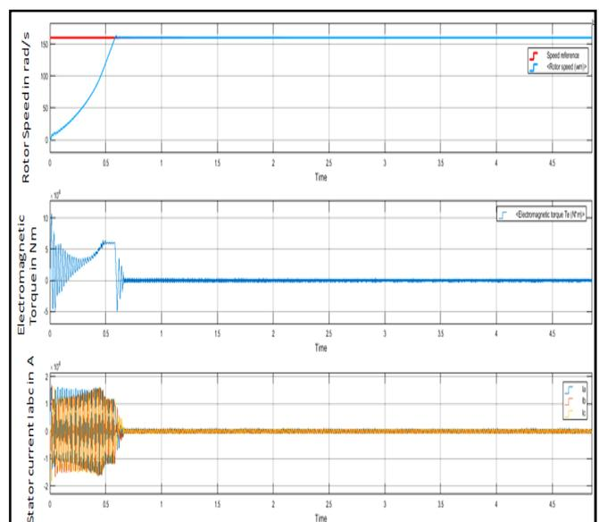
Fig-5: Performance of DFIM drive system when given reference speed is 160rad/sec at no load.
