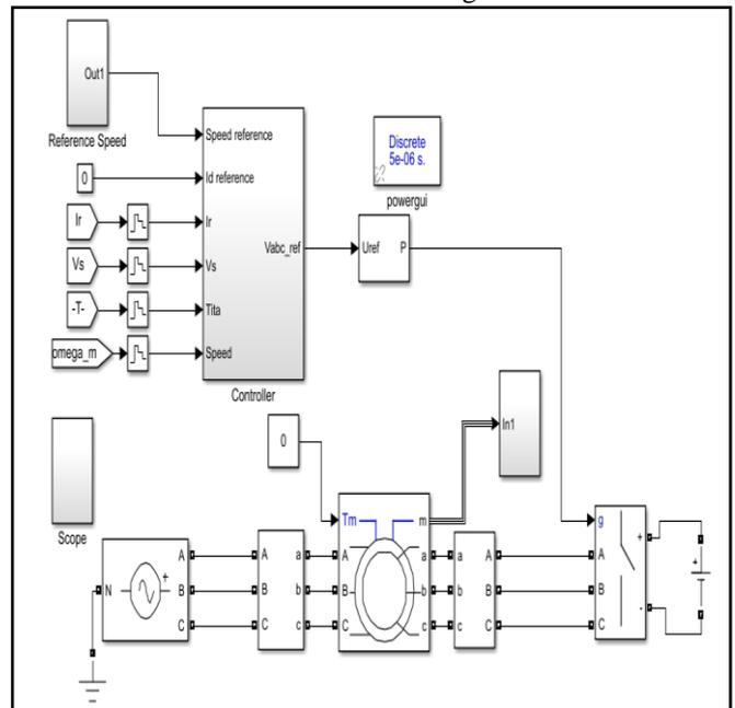
Fig-4: Simulink block diagram of Vector control of DFIM
