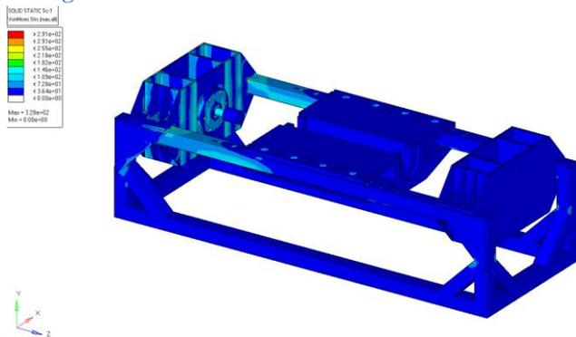
Figure 9 Stress counter of machine
