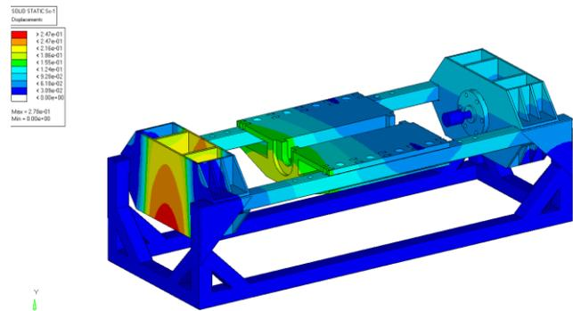
Figure 6 Deformation Counter of Machine
