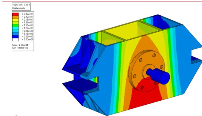
Figure 8 Deformation Counter of Press machine
