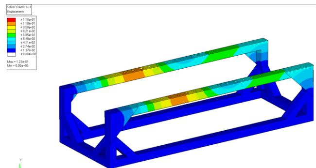
Figure 7 Deformation Counter of Frame
