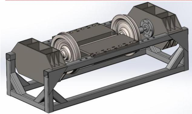
Figure 2 CAD MODEL OF PRESS MACHINE
