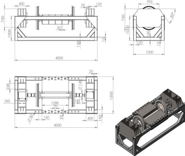
Figure 3 Dimension of CAD Model
