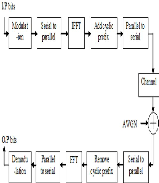
Figure 2. Block diagram of orthogonal frequency division multiplexing transmitter and receiver.
