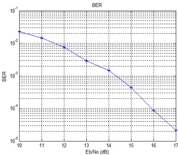
Figure 6. Plot of bit error rate versus  $E_b/N_0$  for  $E_b/N_0$  from 10 to 20 dB using binary phase shift keying.
