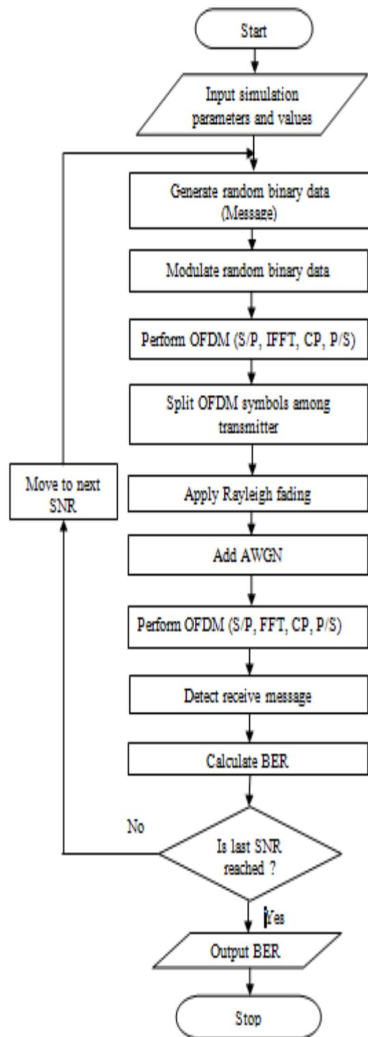
Figure 3. Flowchart for bit error rate calculation in multicast multiple input multiple output system.
