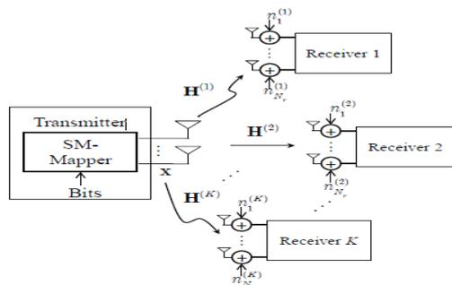
Figure 1. System model of multicast spatial modulation type multiple input multiple output system, adapted [11].
