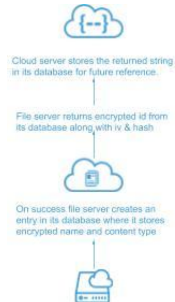
Figure 2: Cloud Server Stores the Reference returned by file server in response after storing the file securely .
