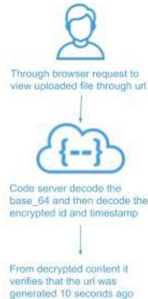
Figure 4: Code Server verifying the .url which is trying to access the resource.
