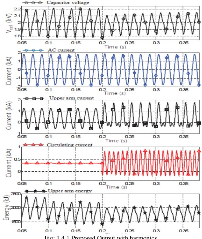
Fig: 1.4.1 Proposed Output with harmonics
