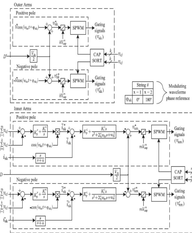
Figure: 1.3.4 Proposed control loop each string is compensated by SVPWM.
