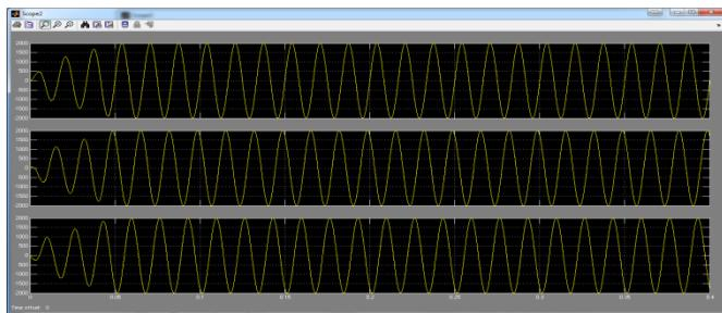
Figure: 1.4.3 proposed system Current waveform after controlling of harmonics
