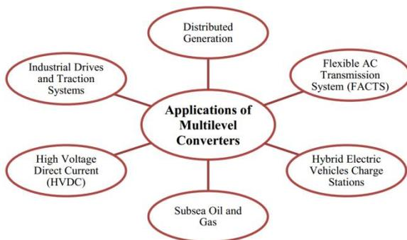
Figure: 1.1.2 Application of Multilevel Converter
