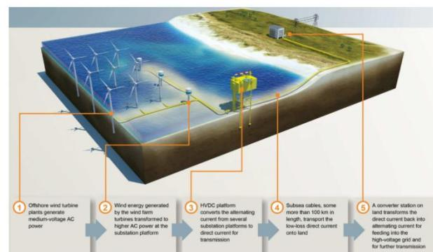
Figure: 1.1 HVDC transmission systems from an offshore to onshore grid.
