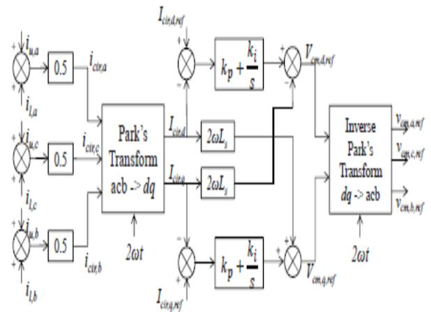
Figure: 1.3.3 Existing control loop only P – Q compensation.
