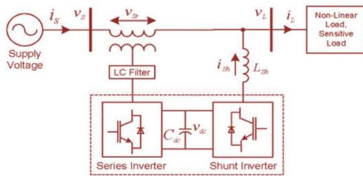
Fig. 2.1 The circuit diagram of the unified power quality conditioner.
