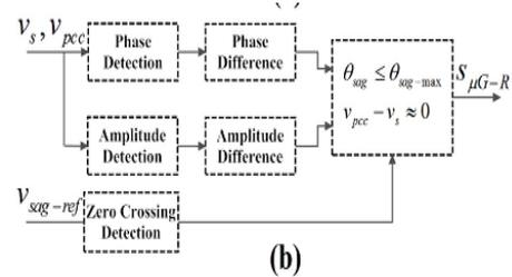
Fig.3.3. (a) Position of  $V_s$  and  $V_{pcc}$  for different phase differences to measure the V sag and  $V_{sag-ref}$ . (b) SynRec  $\theta_{sag-max}$  can be found as
