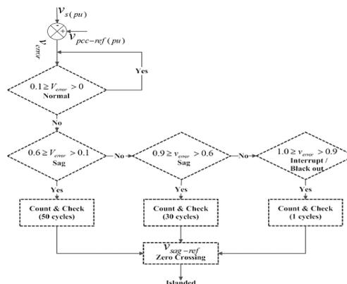
Fig.3.2. Algorithm for Is D method in UPQCμG-IR.
