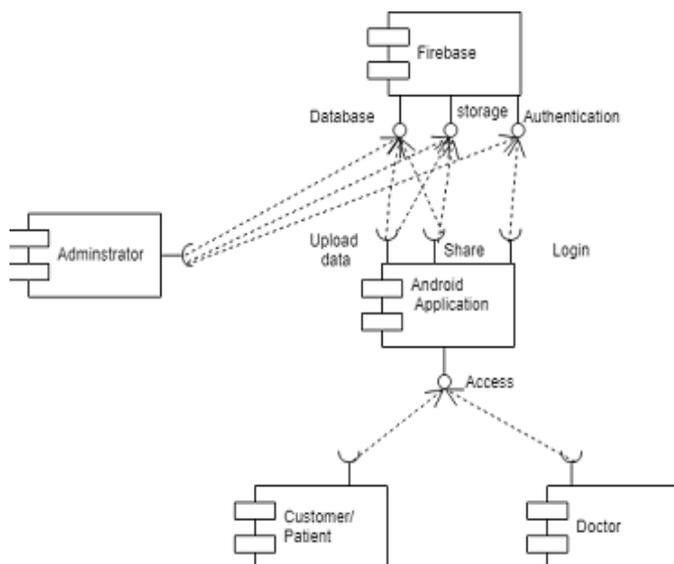
2. Component level diagram for proposed system
