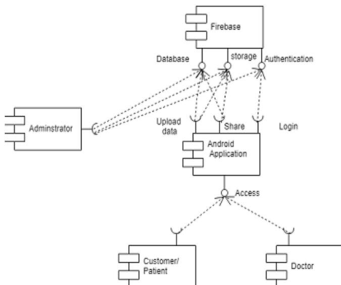
2. Component level diagram for proposed system
