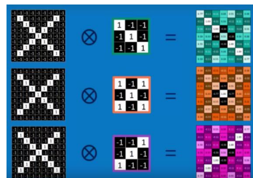
Figure 3. Convolution of each filter with all image matrices to obtain various feature maps
