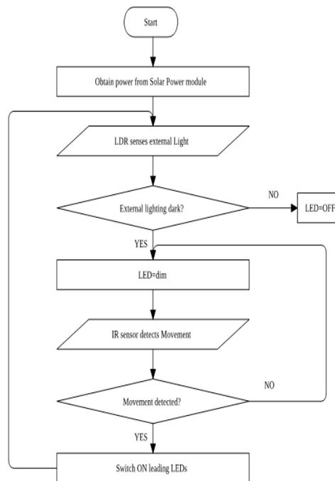
fig. (ii) Implementation flow of the proposed system
