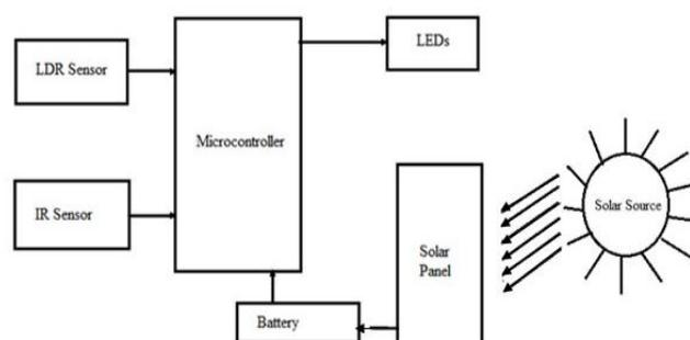
fig. (i) Block diagram of Movement Sensing Street Lighting
