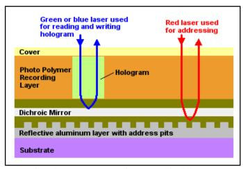
Fig-4: internal structure of Holographic disk[8]
