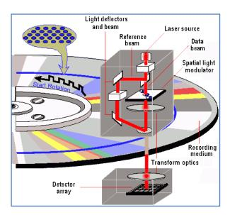
Fig-1:working of holographic disk[7]
