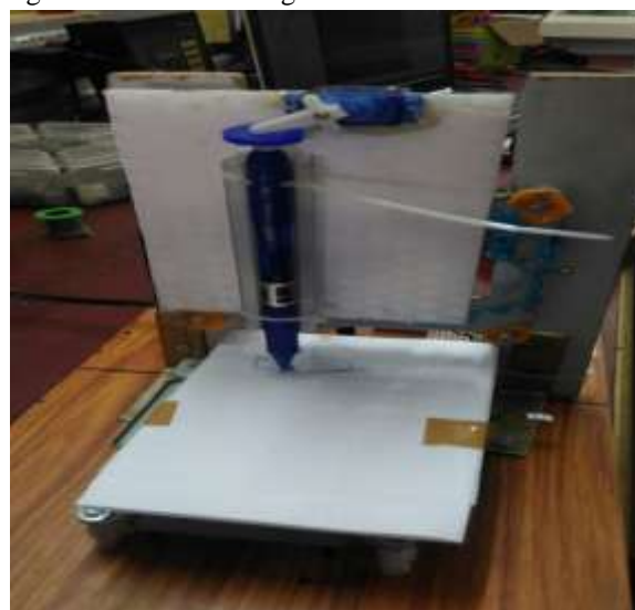
Figure-3: Implementation of 2D- CNC Plotter
