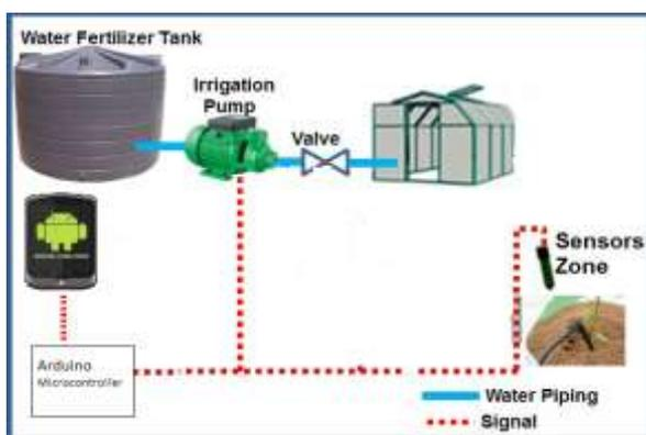
Figure 1: Proposed Irrigation Layout
