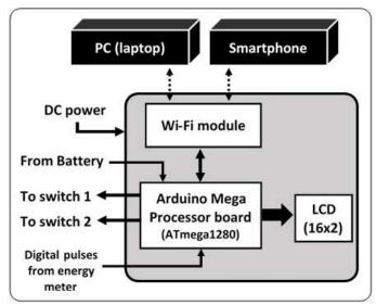
Fig.:2Arduino MEGA is used as an embedded systemand connection with wireless LAN module
