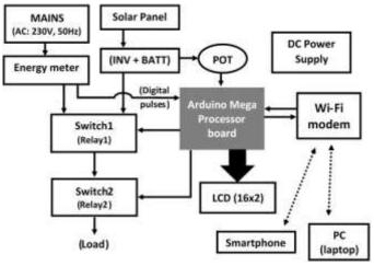
Fig.:1 Block diagram of the system
