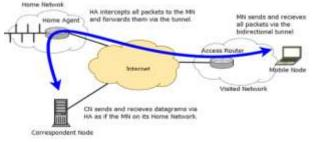
Figure 2: Operation of Mobile IPv6 with Bidirectional tunneling.
