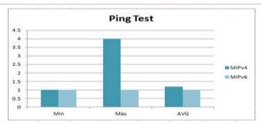
Figure 12: MIPv4 and MIPv6 round trip times in milli-seconds.
