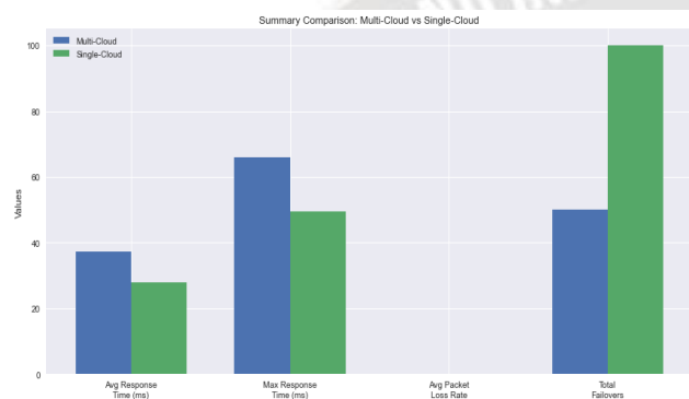
Figure 10: Comparison of Average response time, max response, average packet loss, total failures.
