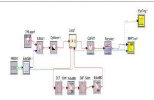
Figure 2 Simulation setup of an optical communication system consisting of DCF for nonlinearity mitigation
