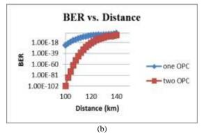
Figure 4 Comparison of an optical system consisting of One OPC and Two OPC (a) Q-factor vs. Distance and (b) BER vs. Distance
