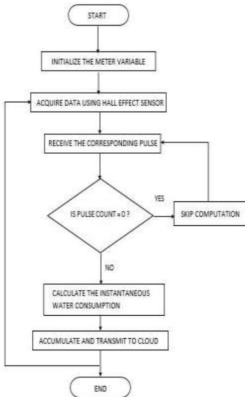
Figure 2. Process Flow
