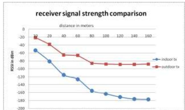
Figure 7. Signal strength -range analysis of receiver
