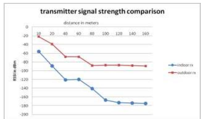
Figure 8. Signal strength -range analysis of transmitter
