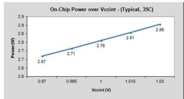
Fig 8(j). Graph showing power consumption of proposed ALU design
