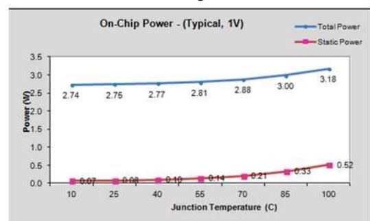
Fig 8(j). Graph showing power consumption of proposed design w.r.t. junction temperature
