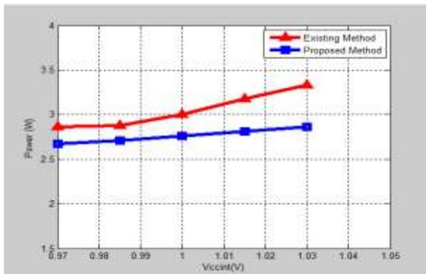
Fig 8(i). Graph showing comparison of power consumption of existing design[7] and proposed design
