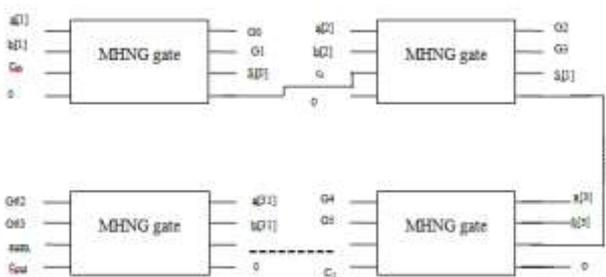
Fig 4. 32-bit Reversible Full Adder Design
