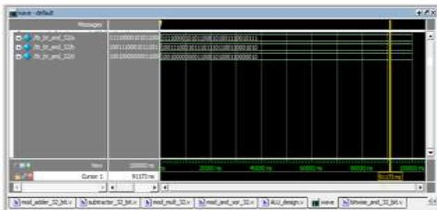
Fig 8(d). Simulation result of 32-bit AND operation
