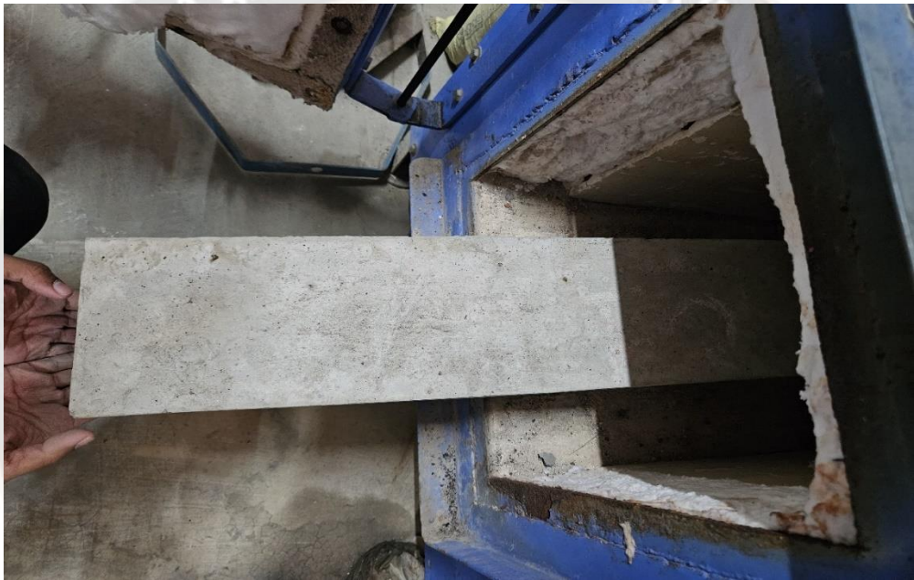
Figure 9: Fired Process on Beam At (500°)
