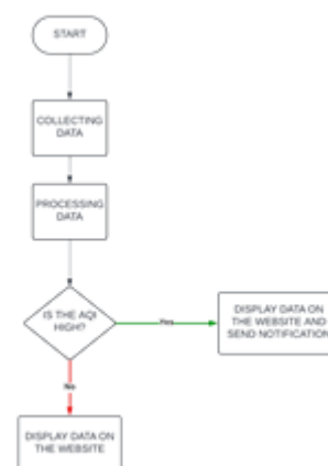
Figure 7. Flowchart of the AirWatch monitoring system
