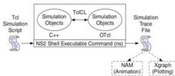
Figure 4: Basic architecture of NS2 [2]
