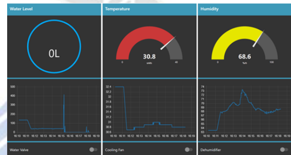
Figure 6. Dashboard of the smart monitoring system (water level, temperature, and humidity).
