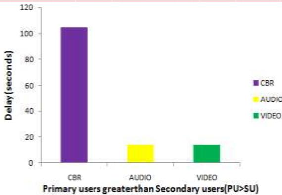
Figure 13. Delay when the traffic is CBR, Audio and video where  $PU_s > SU_s$
