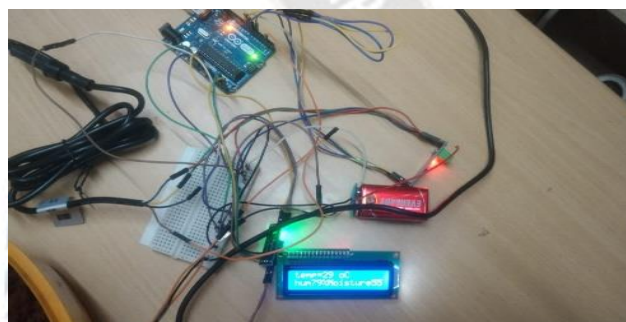
Figure 3 LCD displaying temperature, humidity, Soil Moisture.
