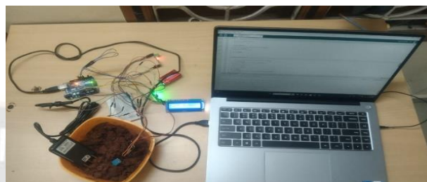
Figure 2 NPK, Temperature, Moisture sensor connections with Arduino and LCD
