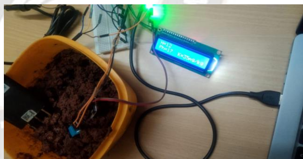
Figure 4 LCD displaying Nitrogen, Phosphorous, Potassium values in mg/kg
