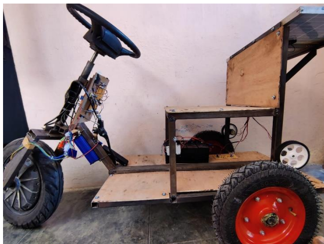
Fig 3: Output of solar and dynamo powered EV using Fingerprint authentication.
