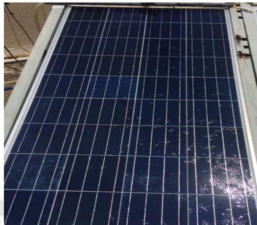
Figure 4.1 Front Surface Cooling by water
