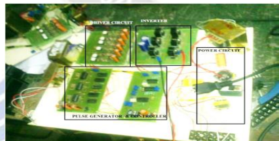
FIGURE 13 TOP VIEW OF THE HARDWARE
